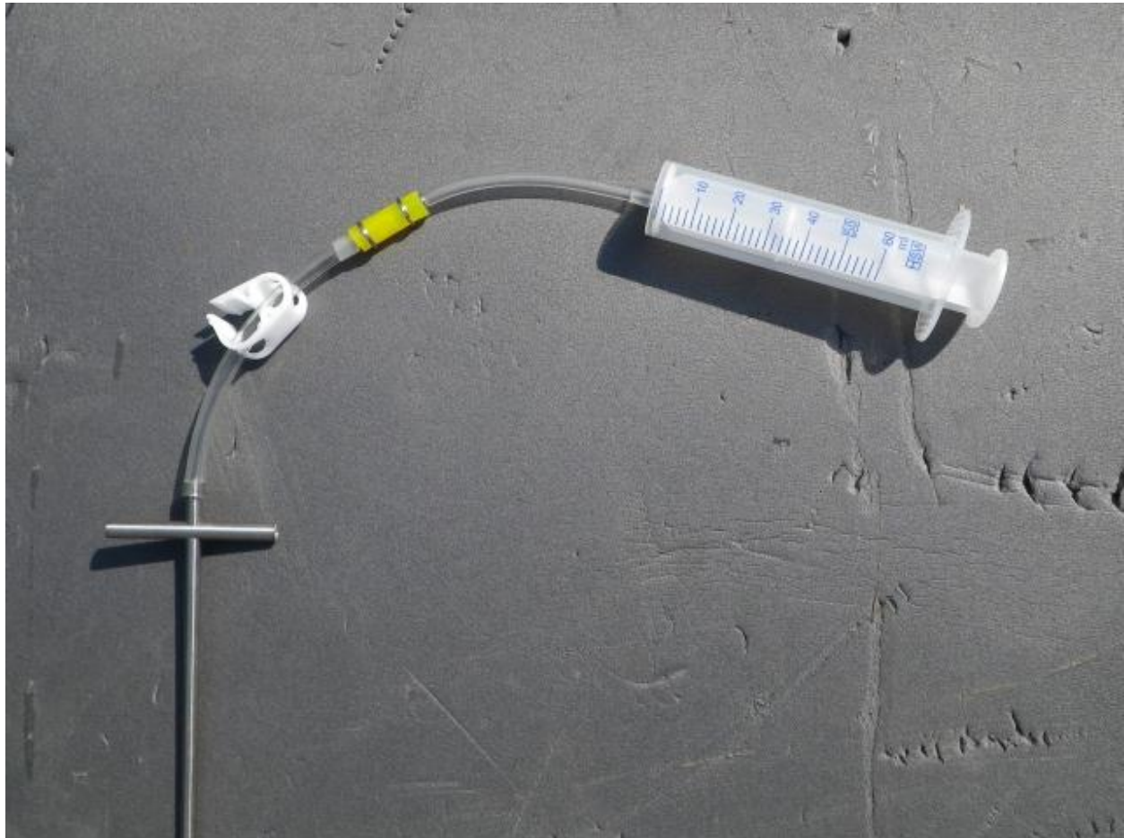
Figure 3: Pinch Clamp connection to a \frac{1}{4} " Syringe Assembly using a 1" piece of \frac{1}{4} "OD polyethylene
