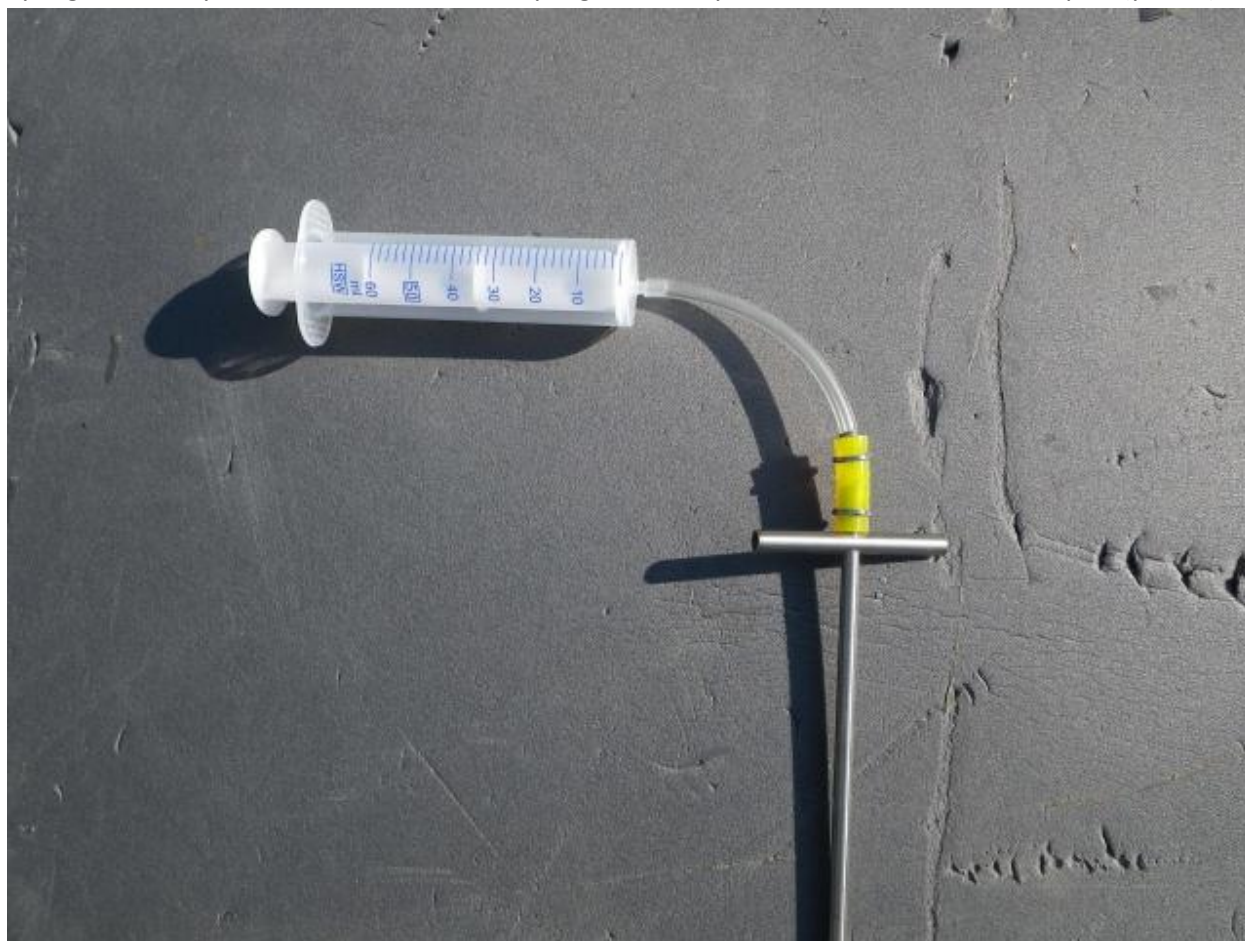
Figure 1: ¼" Syringe Assembly connected to a ¼" diameter PPX36 PushPoint Sampler
