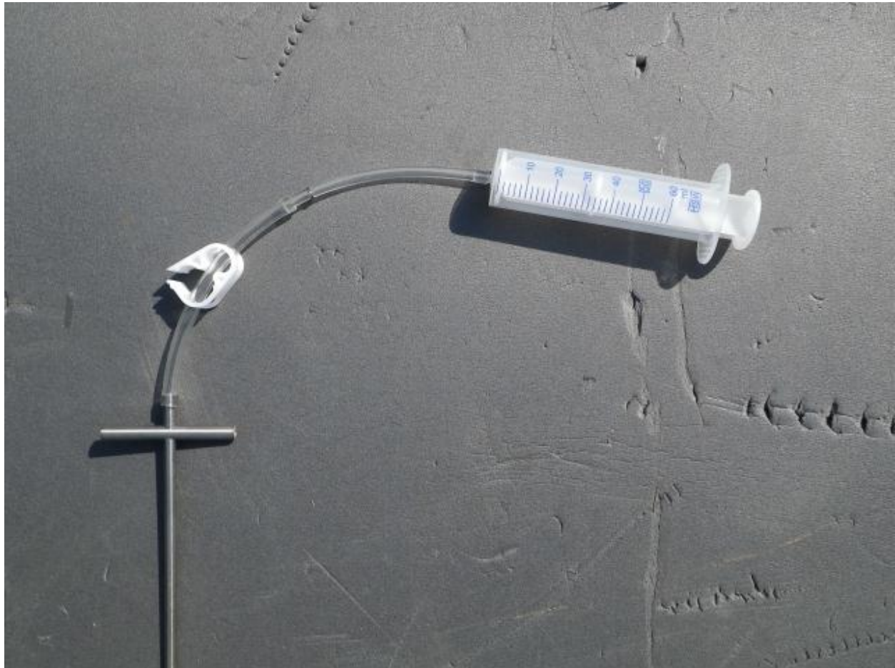
Figure 2: Pinch Clamp connected to 1/8" Syringe Assembly
