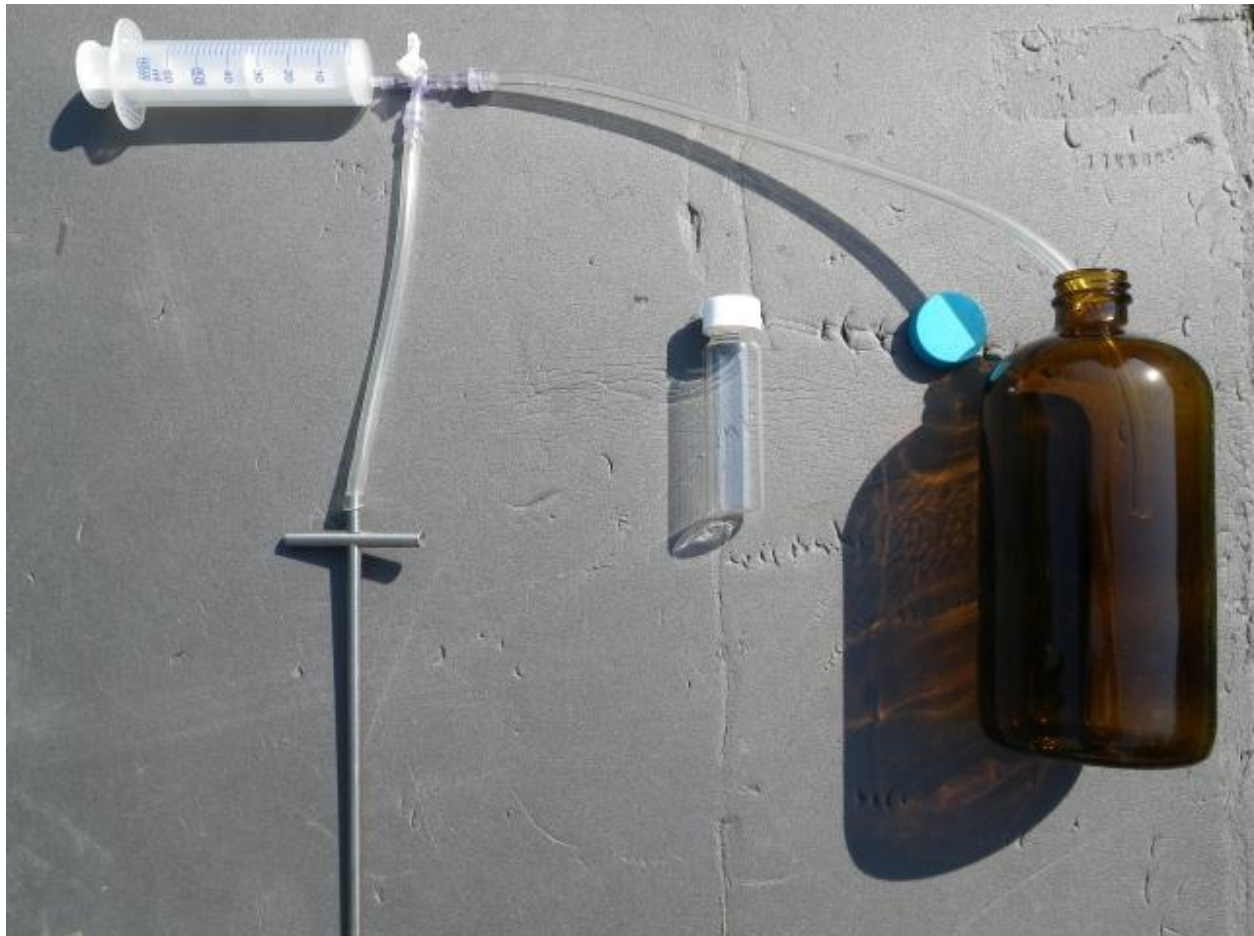
Figure 4b: SyringePump setup for filling 40 ml VOA vial or 1 L Amber bottle.
