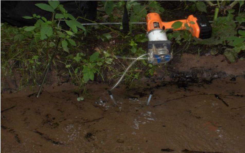
Figure 4: Two SedPoints installed at 5.5' and 3' below the sediment surface. A portable DrillPump (MHEproducts.com) is used for sampling.
