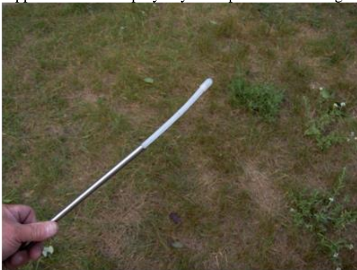
Figure 2: SedPoint w/ polyethylene tip partially loaded into installation tool.
